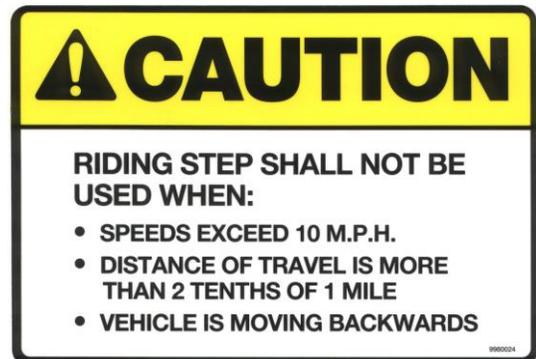
THIS DECAL WARNS OF THE HAZARD OF RIDING ON BACK OF THE VEHICLE. THE VEHICLE DRIVER CAN NOT ACHIEVE VISUAL CONTACT (USING MIRRORS) IF HIS WORK PARTNERS ARE BEHIND THE VEHICLE, IN THE BLIND SPOT.
