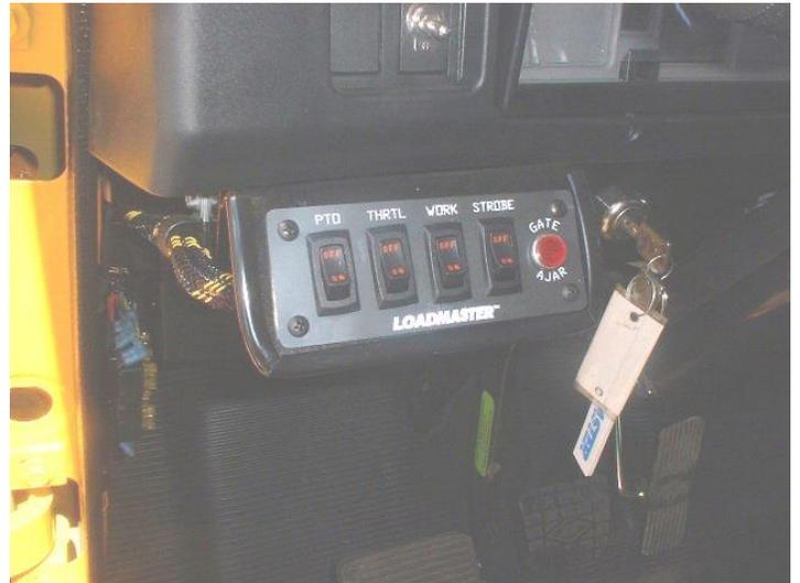
**Turn on your beacon or strobe lights (and the hopper area work lights, if needed)** by positioning the rocker switches so that the red band is exposed.
