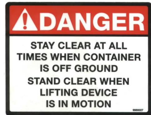
THIS DECAL WARNS OF THE HAZARD THAT WILL OCCUR IF THE CONTAINER'S TRUNNION BARS ARE NOT SECURELY CAPTURED ON **BOTH SIDES** BY THE "LATCH ARMS" DURING CONTAINER DUMPING. THE CONTAINER TRUNNION BAR COULD DETACH COMPLETELY OR PARTIALLY FROM THE TRUCK-MOUNTED COUPLER AND MOVE UNCONTROLLABLY CAUSING INJURY.
